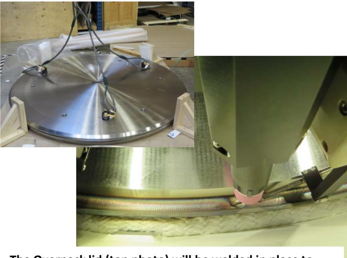
The Overpack lid (top photo) will be welded in place to provide a secure shipment-ready package.
