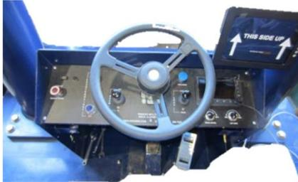
The operator’s control station contains interfaces for all functions of the TL220 and a real-time display of vital equipment information.
