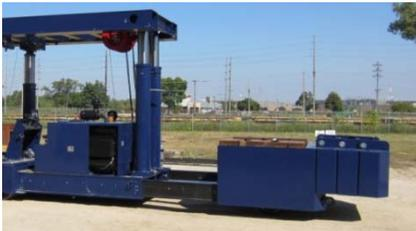
Robust hydraulic cylinders (middle photo) and extendable rear counterweights (above) will accommodate heavy lifting.
