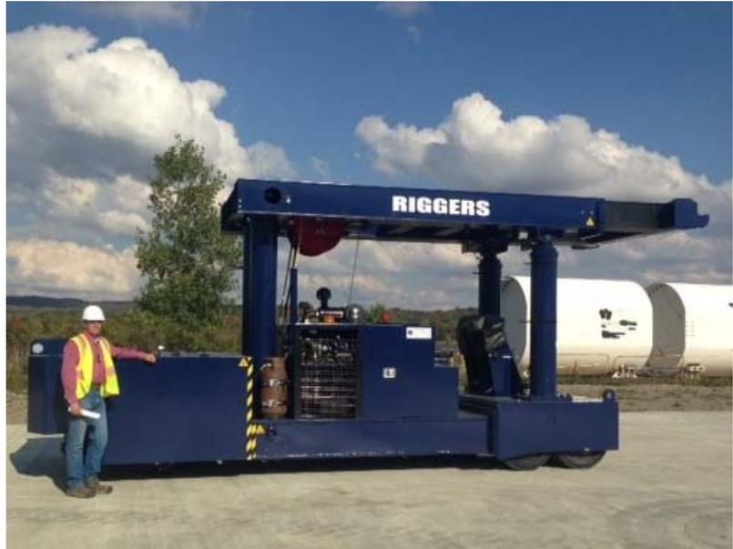
The TL220, pictured above, is one of three transporters that were specially-designed for lifting and moving HLW storage casks.
