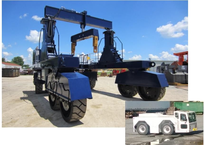
*The Vertical Cask Transporter (top photo) that will be used for outdoor transport of HLW storage casks at the West Valley Demonstration Project and the tow tractor that will pull it are pictured above.*
